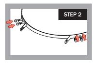
on the bottom ceramic grill body with bracket slots facing up. Brackets are stamped on the back with letters indicating their position (e.g., **LF**=Left Front bracket and **RB**=Right Back bracket). Mount a flat washer then acorn nut on each stud and tighten with provided wrench.
